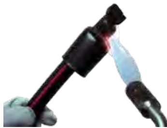
2. Beginning at closed end apply heat, blue thermochromatic lines will begin to disappear at 150° C. Gradually, move heat source to open end and around cap. Once lines are no longer visible and adhesive flows out of open end, discontinue heating.
