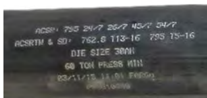
Above: close up of marking on Fargo splice requiring 14SH die index.
